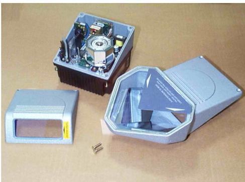
2. Mount the GFX-60 onto the scan head paying attention to correctly align the sealing gasket.
