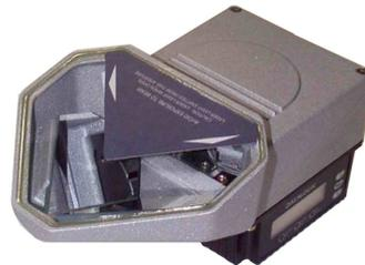
6. Mount the scanner at an angle of  $16^\circ$ , as indicated in figure below, in order to obtain an angle of  $90^\circ$  between the two scan lines. This guarantees an omni directional reading of the barcode, if the code label satisfies the ACR3™ conditions (see Scanner Reference Manual for details).
