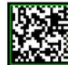
Quiet zone violation
