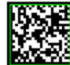
Quiet zone violation
